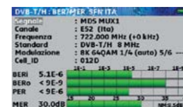
Misure di bBER, aBER, UNC, BER, PER, Noise Margin
